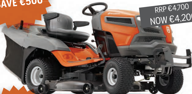
HUSQVARNA TC 342T Kawasaki V-Twin, 13.3 kW@2600 rpm, Hydrostatic, 107 cm, LED headlights.
